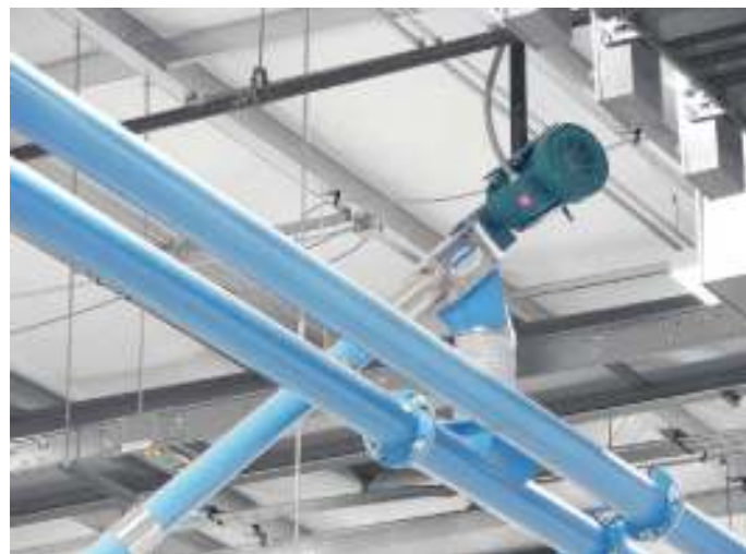
ABOVE: Helix flexible screw conveyor feeding into tubular drag conveyor
