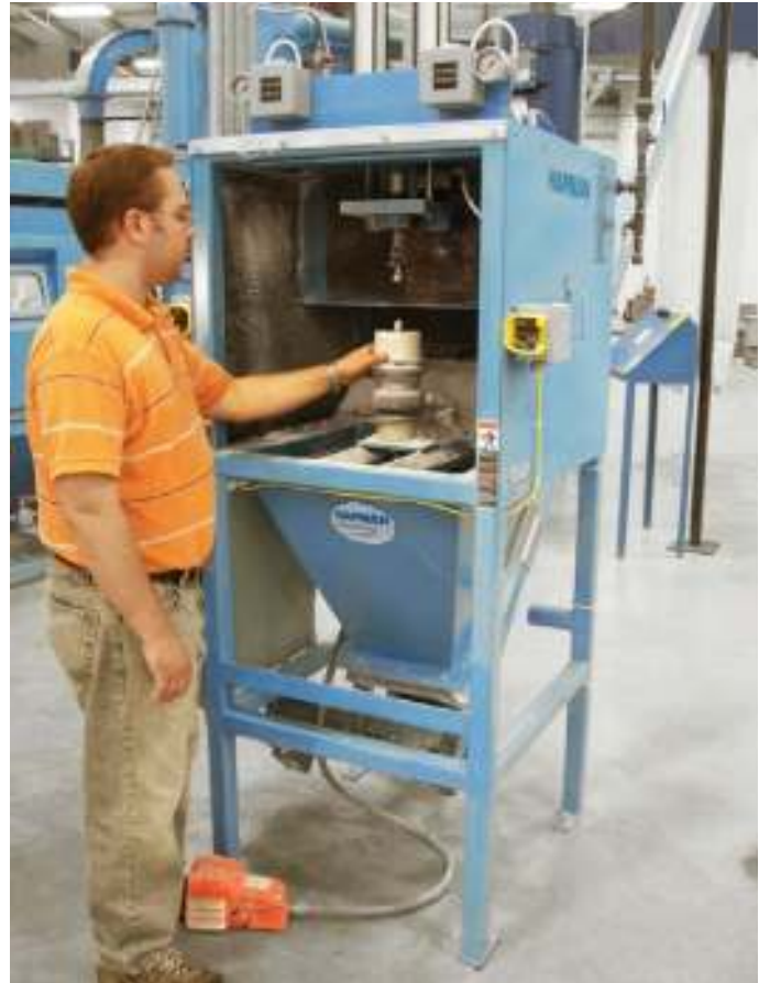
ABOVE: Knock out station with specially designed apparatus and integral dust hood
