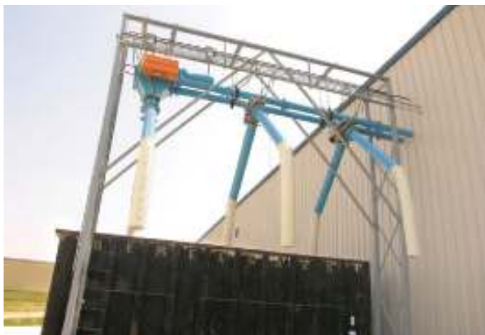
ABOVE: Discharge end. Each discharge has a bi-directional gate
